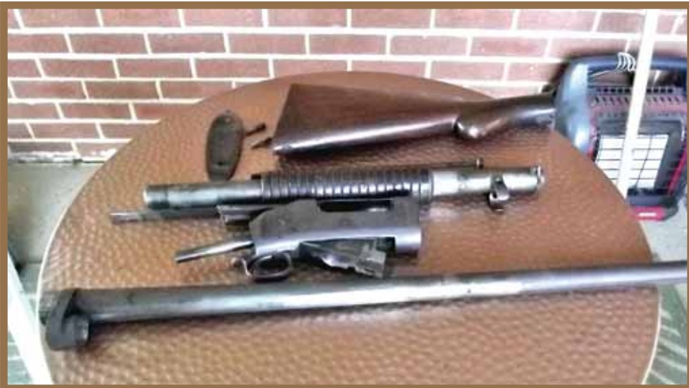
Top Left Photo: The only problems with disassembly was the rusted and frozen barrel band screws. I don't think the picture shows the extent of the exterior rust very well. The color of the table blends into the color of the rust. Top Right Photo: My experience has been that when the toe of the stock cracks and comes apart from the rest of the stock it's due to someone tightening the butt plate screw that is to large for the hole and expanding the wood causing it to crack along the grain of the wood. Bottom Right Photo: The bore had a fine layer of rust but cleaned up nicely. There was a layer of leading which indicated to me that the gun had a lot of use over the years. (Author Photo)
