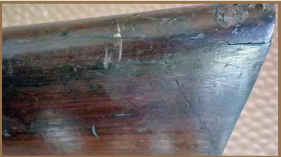
Top Left Photo: The only problems with disassembly was the rusted and frozen barrel band screws. I don't think the picture shows the extent of the exterior rust very well. The color of the table blends into the color of the rust. Top Right Photo: My experience has been that when the toe of the stock cracks and comes apart from the rest of the stock it's due to someone tightening the butt plate screw that is to large for the hole and expanding the wood causing it to crack along the grain of the wood. Bottom Right Photo: The bore had a fine layer of rust but cleaned up nicely. There was a layer of leading which indicated to me that the gun had a lot of use over the years. (Author Photo)
